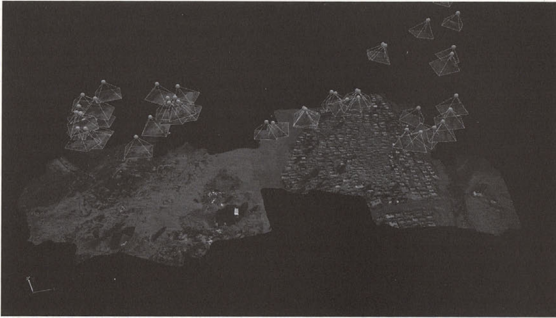
Model showing the locations of photographs taken by a kite-mounted camera in the Negev Desert. Forensic Architecture (Ariel Caine) and Public Lab (Hagit Keysar).
