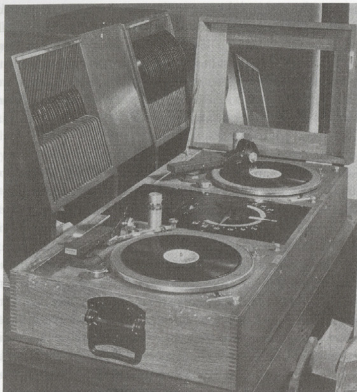
Figure 29.4. Western Electric Non-Sync Turntable Unit, ca. 1929. (Source: F. H. Richardson, Handbook of Projection , 5th edn, Vol. 3 (New York: Chalmers Pub Co., 1930).
